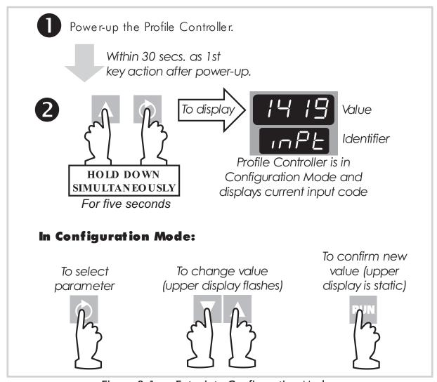
Figure 3-1 Entry into Configuration Mode
